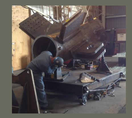
Work Proceeding at Oregon Ironworks – robot welding, cast node with attachment plates, cast node attached to pipe column.
