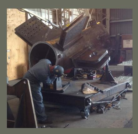
Work Proceeding at Oregon Ironworks – robot welding, cast node with attachment plates, cast node attached to pipe column.
