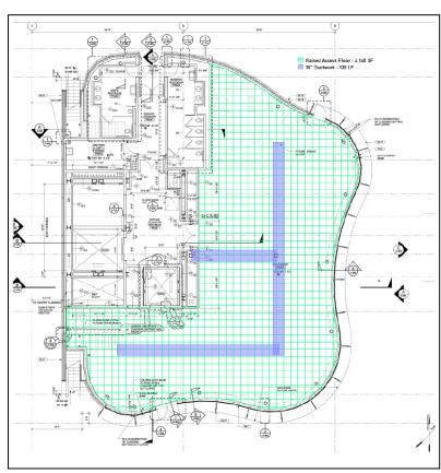
Space Plan, showing ducting and floor area
